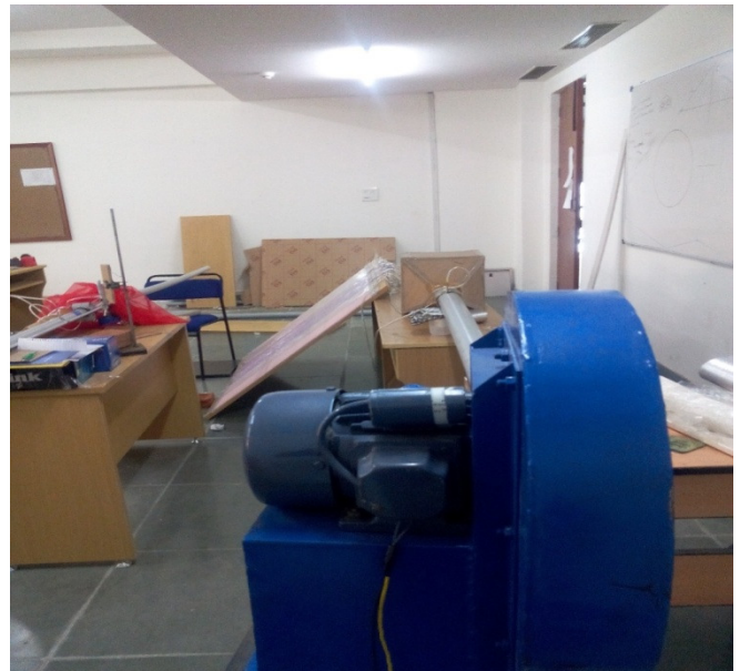
Fig. 6. Experimental Setup of Rectangular Duct with Inverse Ratio.
